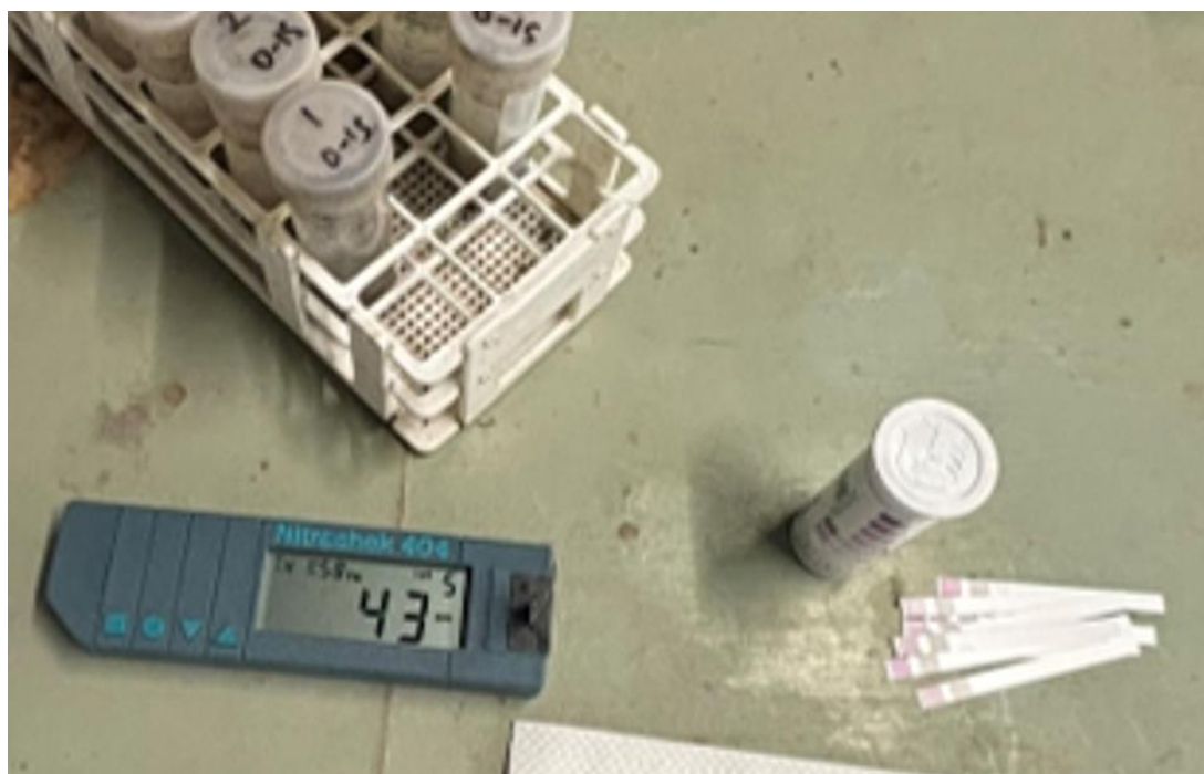
Figure 2-2 Nitrachek 404 method components showing the electronic reader, MQuant test strips, and test tubes used for extraction in the soil nitrate testing process.
