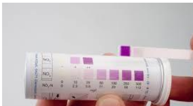
Figure 1-1 Comparing a test strip against the colour matrix on the test strip container.
