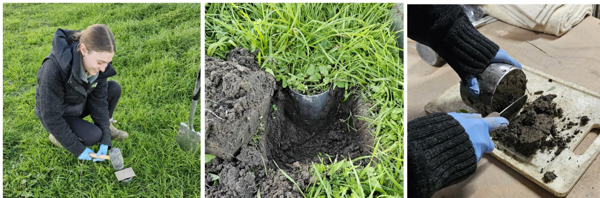
Figure 2-1 Bulk density sampling procedure showing (left) bulk density ring insertion, (centre) soil core extraction, and (right) sample preparation for oven drying.
