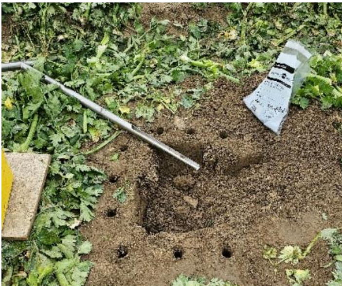
Figure 2-4 Ten soil cores were taken around the VSA hole and sent for laboratory testing to determine the total carbon concentration.
