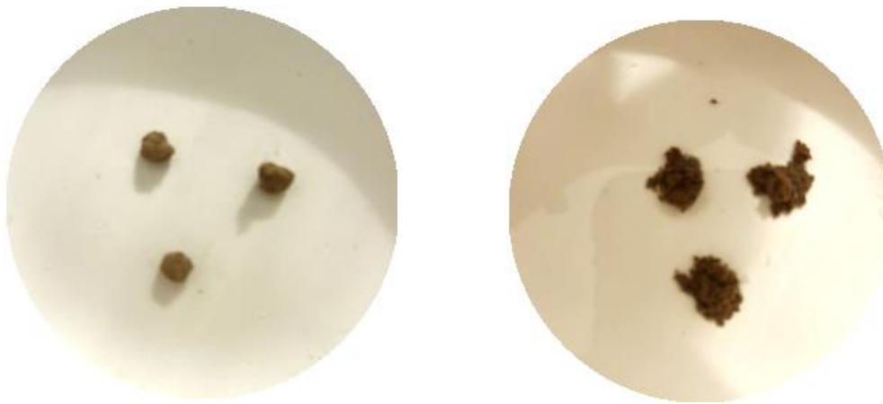
Figure 2-2 Left: Initial photo of the dry aggregates taken by the Slakes app. Right: Final photo taken automatically by the Slakes app ten minutes later.
